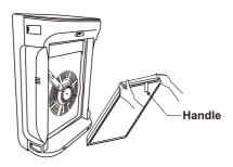
Step 3: install the filter screen in the specified direction;
