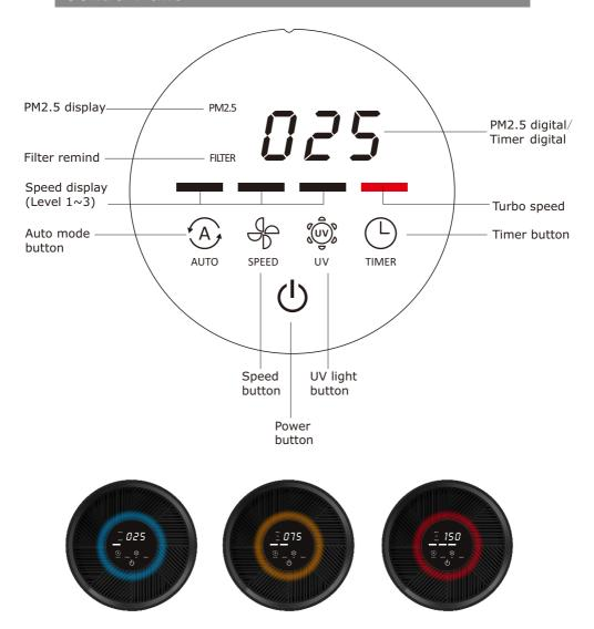
The indicator Lamp will light up, the Ring Lamp will light up in corresponding colors on the basis of air quality.
