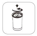
2. Turn the bottom cover counterclockwise and remove the filter;
